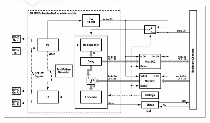
The SDI standard defines up to 16 audio channels transmitted within a video signal. These 16 channels are divided into four groups of four channels each. Selection of which channels are to be embedded or de-embedded is performed by DIP switches on the card (or by software, if supported): either groups 1&2, groups 3&4, or all.
