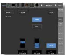
To compensate for audio to video signal offsets when operating the OnAir 3000 in a TV environment, systems using the SCore Live DSP core enable a delay function. During operation, delay can be activated on input channels, master and aux busses, N-x and subgroups. It is possible to set any delay time between 0 and 5 seconds in a resolution of milliseconds.
