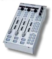
The Editor Module is an extended three-fader module including a subset of monitoring and talkback functionality and buttons for the assignment of the rotary function. Eight freely configurable buttons each for monitoring source selection and talkback destination, four configurable buttons for rotary functions like input routing, gain, etc. and volume control for editor headphone, guest headphone and loudspeaker volume allow for a standalone working environment, e.g. for a journalist or editor.
