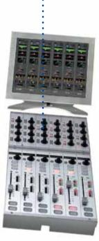
Modules of three or six faders can be added up to a total of 48 faders if required. The fader strip includes input level metering, five freely configurable push buttons, a rotary encoder and an alphanumeric display. Using only the fader modules and fader screens gives the operator an excellent overview of the console while presenting a very clean surface with the minimum necessary elements.
