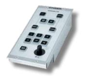
The Surround Control Module is an extension to the existing Monitoring and TB Module. The user can easily switch between Internal Stereo Mixdown and External Stereo Encoder (e.g. DOLBY®), mute individual speakers and switch to an alternative Stereo Nearfield speaker set with its own dedicated volume control rotary.
