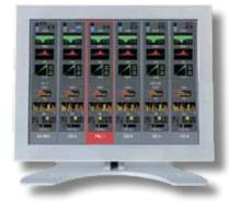
The colour 12" touch sensitive fader screens display the input settings, equalizer and dynamics settings, AUX send levels, N-X contribution, input, output and insert routing, bus and group assign, Pan/Bal and channel label, all in real time with real values. The Fader Screen is also available in a multi functional version with additional DVI input and two buttons on the front to switch between the standard channel display and any external video source (600x800).
