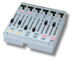
The module contains 6 full 100mm faders, 4 large illuminated and configurable pushbuttons with replaceable label, and 12 small illuminated pushbuttons per channel. Two LED's in each fader strip indicate channel overload (red) and active fader start (blue). Level and gain reduction meters are shown on an OLED display on every channel. Additionally, channel label and channel process parameters are indicated on the OLED as well.
