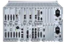
If more inputs or outputs are needed, up to another five external D21m frames may be added to a Compact SCore, or 12 to an SCore Live, and connected to additional DSP cards per D21m frame to the maximum of 6 DSP cards. This results in a theoretical maximum of 576 physical input and 576 output signals. with the Compact SCore, or 1728 x 1728 with the SCore Live.
