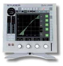
The screen includes a studio clock, two stereo bargraph meters each with phase correlators, two stop watches, menu buttons and eleven freely assignable buttons on the right border of the screen. These buttons can be used in the same way as the buttons in the Fader Assign Module.
